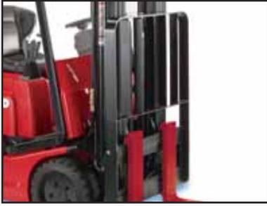
In certain environments of use, high palletized loads or loads stacked higher than the height of the carriage must be handled. The load backrest is an extension of the carriage height and serves to stabilize and provide additional support for such loads. As a consequence, the expanded load backrest extension assists in preventing material from falling and reduces load damage.
